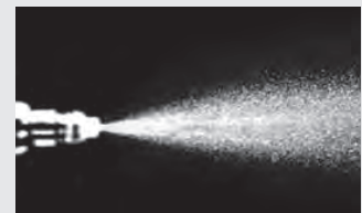
Injector spray pattern after P.i. treatment.
